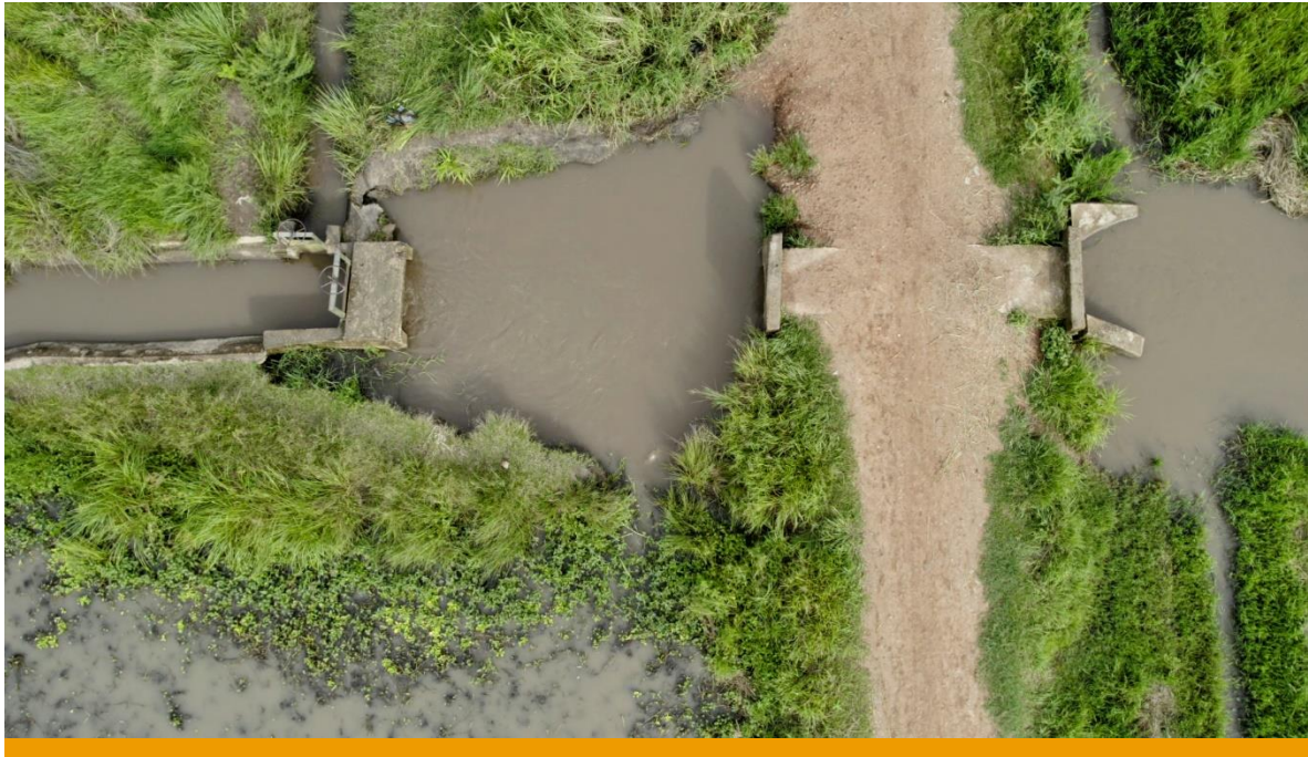
An aerial view of the Tulo Kongwa Irrigation system. The system is unlined, a sign of inefficiency.
