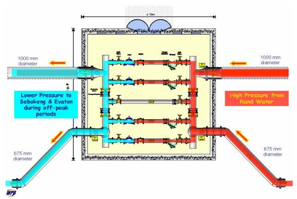
Figure 12. Schematic Representation of the Pressure Management Installation
