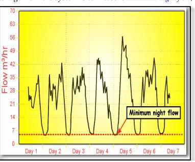
**Figure 5: Minimum Night Flow Where Leaks are Well Managed** (courtesy of Ronnie McKenzie, WRP, Ltd.)
