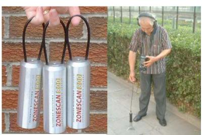
**Figure 6.** Acoustic Loggers and Digital Ground **Microphone for Leak Detection** (Photos: Gutermann International, www.gutermann-uk.com)
