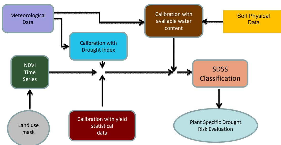
Figure 1. Steps of the process for Plant Specific Drought Risk Evaluation
