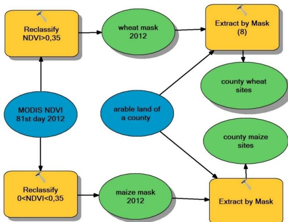
Figure 2. ArcGIS model for creating mask and extraction of wheat and maize site at a ROI
