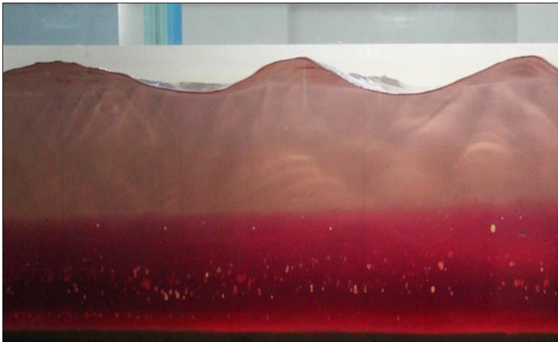
Figure 2.1.1 B Wind, wave and current, salty coupling test tank
