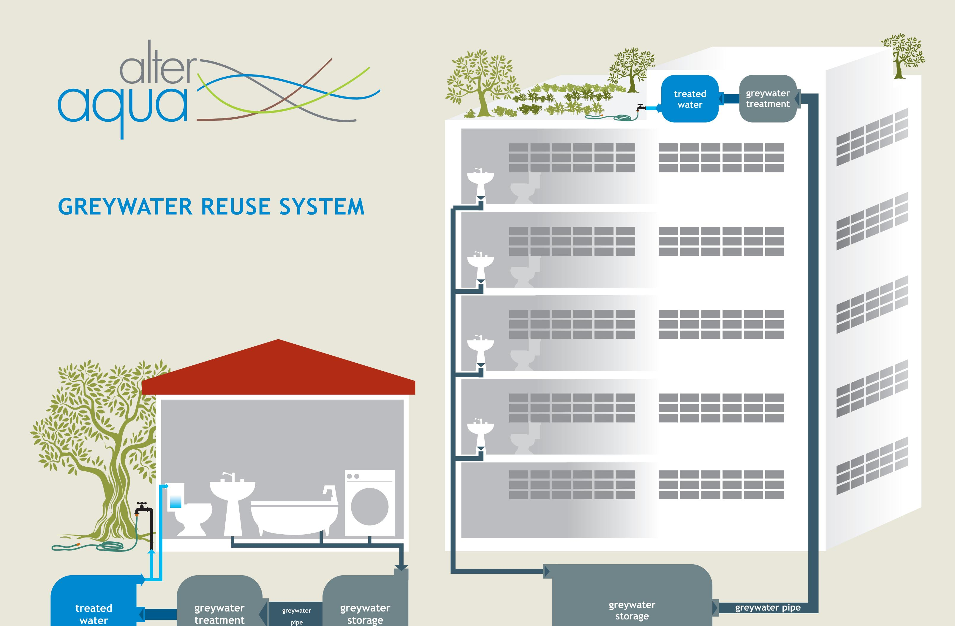
Greywater is defined as wastewater generated from showers, wash basins, washing machines, and partly from kitchen appliances and sinks.
