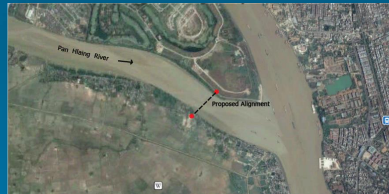
Proposed Alignment of Sluice Gate
