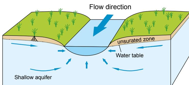
Figure 3.6 : Gaining rivers receive water from groundwater (USGS, 1998)
