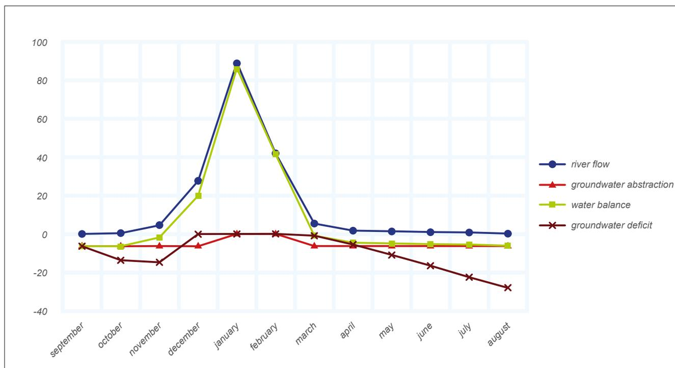
Figure 3: Limpopo chart showing water balance components. Vertical axis is m<sup>3</sup>/sec. River flow line is prior to groundwater abstraction.
