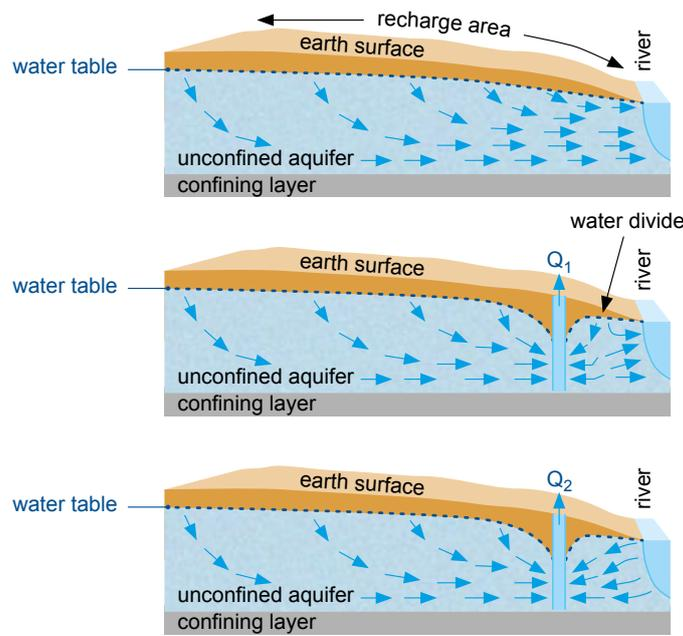
Figure 8.2: Impact of groundwater abstraction on surface water bodies. Natural groundwater flow with discharge to a river (top). Continuous pumping at high rates lowers the water table reducing the aquifer discharge into the river (middle). Excessive pumping leads to a change of the flow situation in which the river water reaches the well (bottom). Source: modified from US Geological Survey
