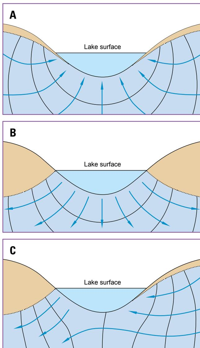
Figure 3.9: Lakes's interaction with groundwater (inflow (A), lose water as seepage to groundwater (B), or both (C))
