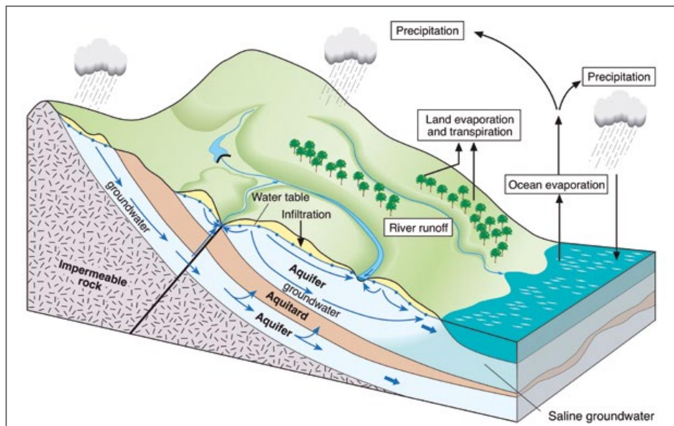
Figure 2.1 Hydrologic cycle: linkages between surface and groundwater.
