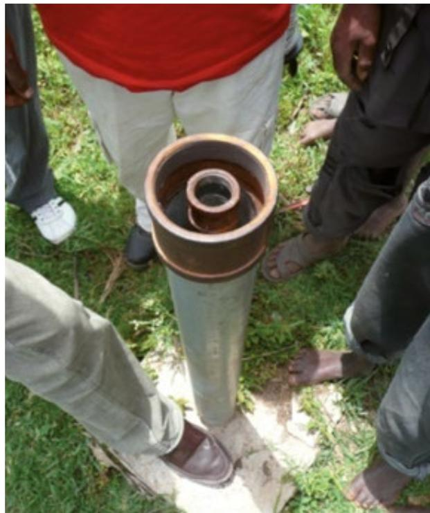
*Figure 5.3 Example of a dedicated monitoring well: a 1" or 2" screen pipe with 3" or 4" upper casing that prevents the wells from flooding and allows for a proper screwed cap for protection. 1" observation wells are for water level recordings only (with a water dipper or a diver). 2" observation wells also allow water sampling with a bailer*
