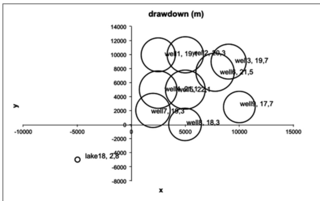
Figure 2. Illustration of interference between pumping wells
