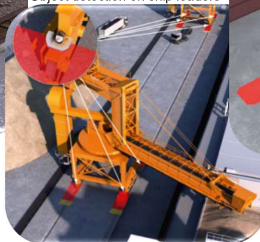
Object detection on ship loaders
