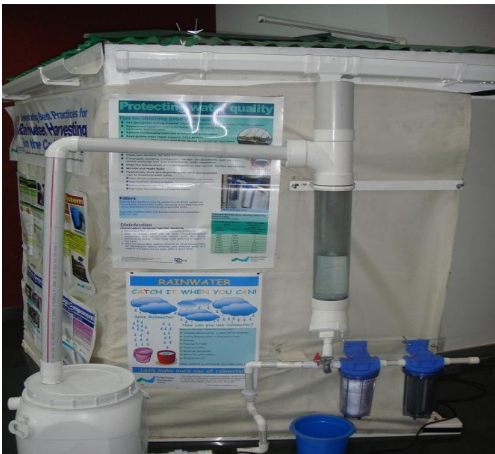
Cross-section of the GWP-C Rainwater Harvesting Model showing the downpipe and first-flush system.
