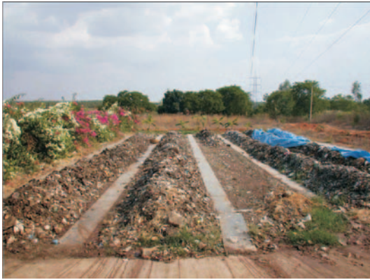
Figure 15. Composting of faeces together with household waste in wind rows. Photo: J Heeb.
