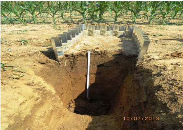
Fig. 6 Water infiltration principle and presentation of infiltrated soil profile
