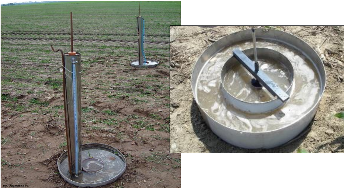
Fig. 10 Infiltrometers installed on the experimental field.
