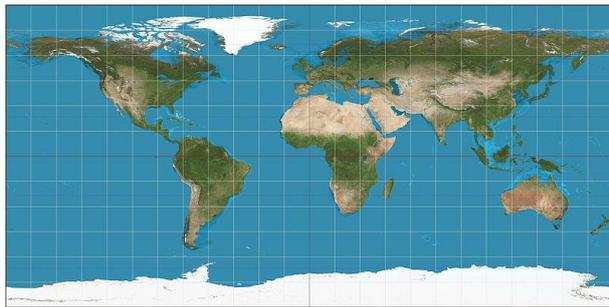
Figure 8: Equirectangular projection (figure from [http://upload.wikimedia.org/wikipedia/commons/thumb/8/83/Equirectangular\\_projection\\_SW.jpg/800px-Equirectangular\\_projection\\_SW.jpg](http://upload.wikimedia.org/wikipedia/commons/thumb/8/83/Equirectangular_projection_SW.jpg/800px-Equirectangular_projection_SW.jpg).)
