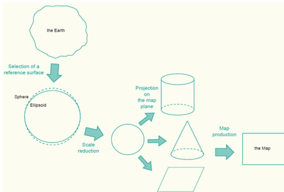
Figure 4: The process of representing the Earth on a flat map (figure from <http://kartoweb.itc.nl/geometrics/Bitmaps/Intro%201.6a.gif>)
