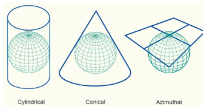
Figure 7: The three classes of map projections: cylindrical, conical and azimuthal (figure from <http://kartoweb.itc.nl/geometrics/Bitmaps/Intro%204.10a.gif>)
