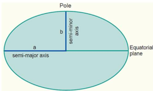
Figure 5: A cross section of an ellipsoid, used to represent the Earth (figure from <http://kartoweb.itc.nl/geometrics/Bitmaps/Intro%201.7a.gif>)
