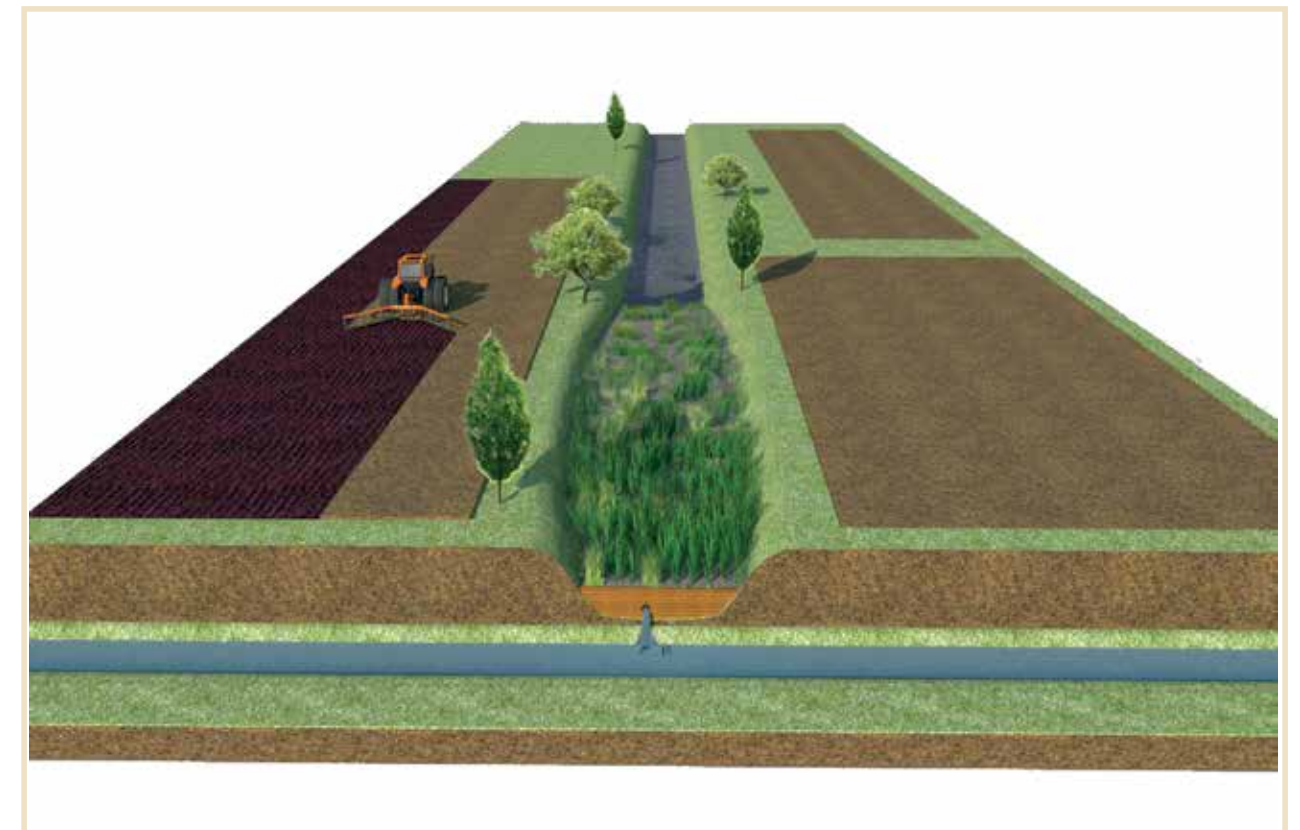
Figure 10. An example of a co-natural system for agricultural run-off treatment.
