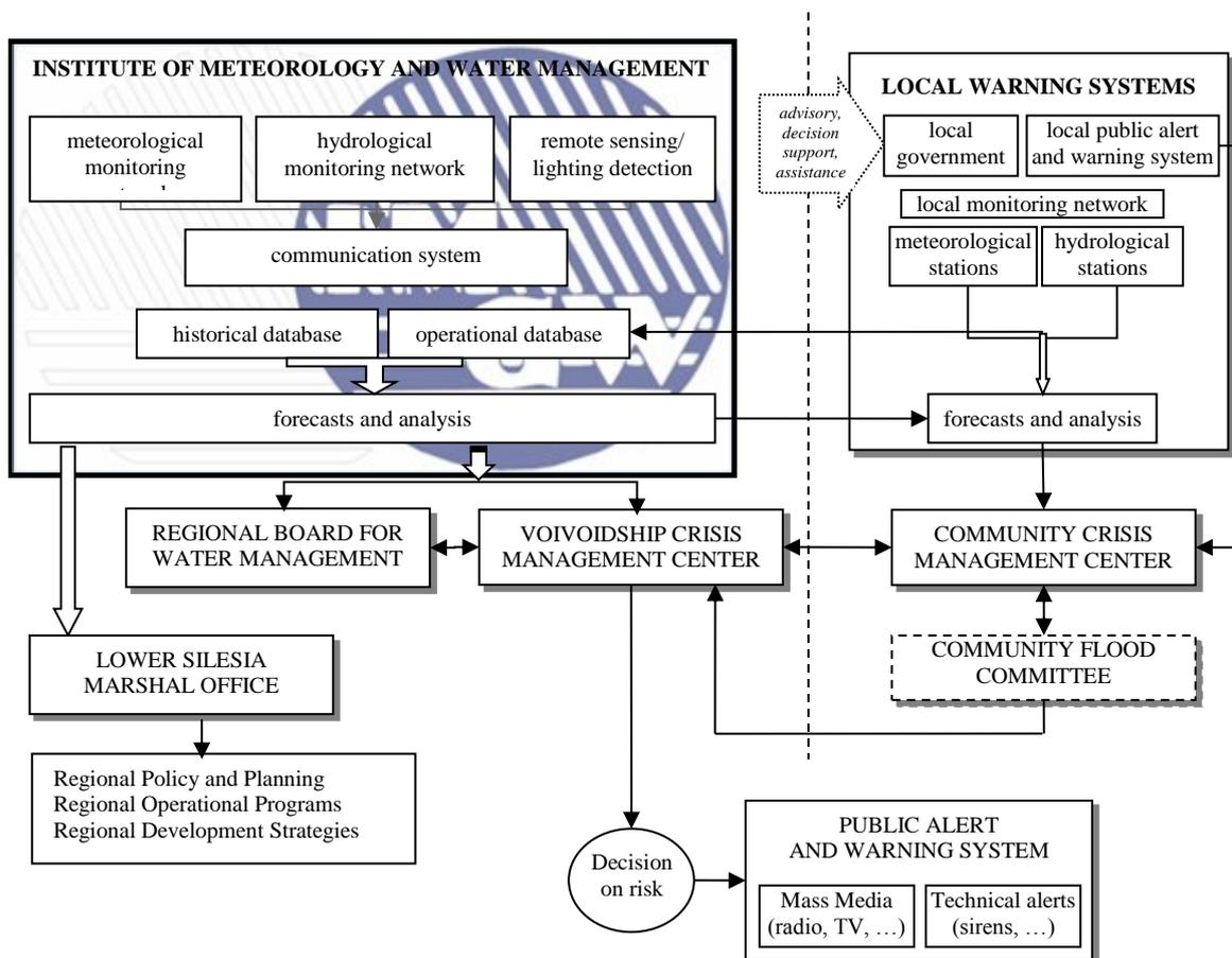
Fig. 4.7.1. Integrated Hydrometeorological Monitoring and Warning System
