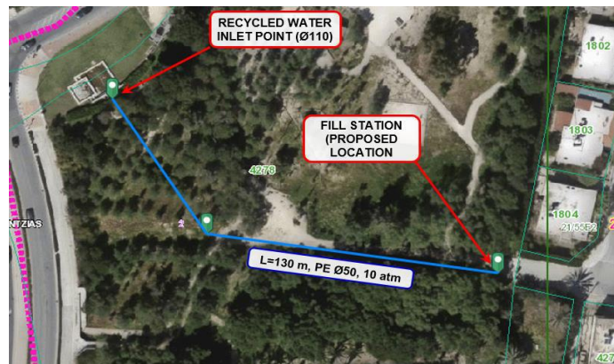
Eukóva 2. Piping between the treated wastewater inlet and the refill station.
