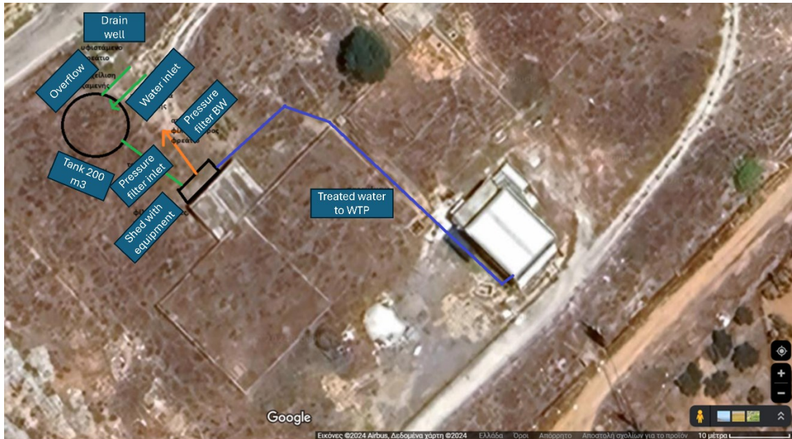
Figure 3. An indicative allocation of the equipment in the WTP area.
