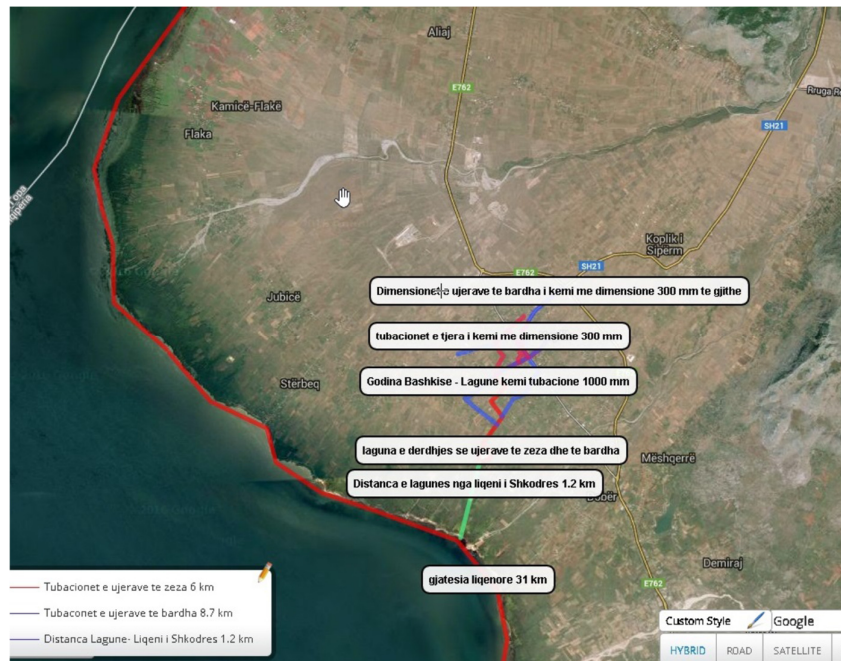
Figure 4: Existing sewerage system in Koplík city
