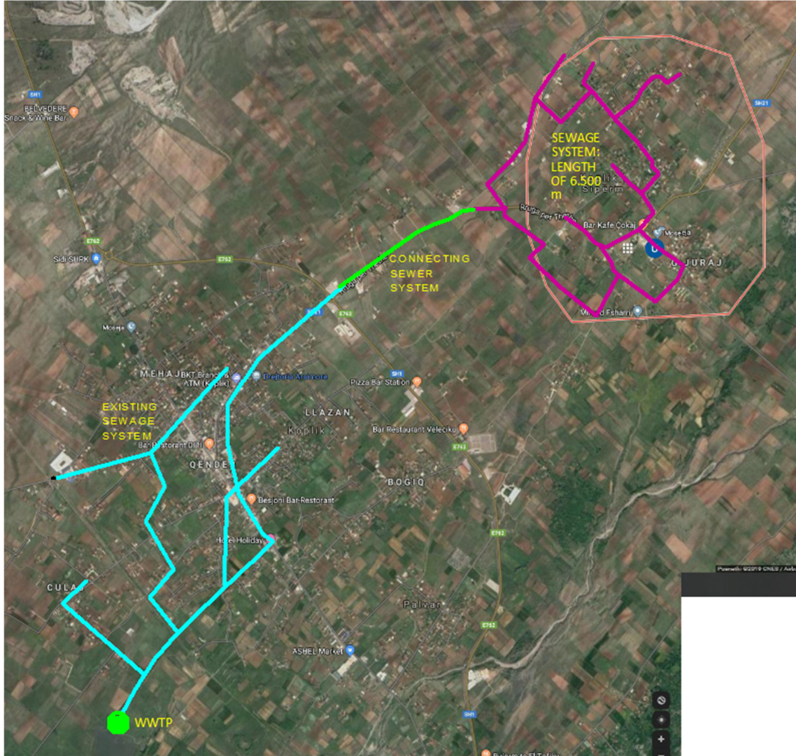
Figure 9: Scheme of the sewer system with WWTP in the village of Koplík
