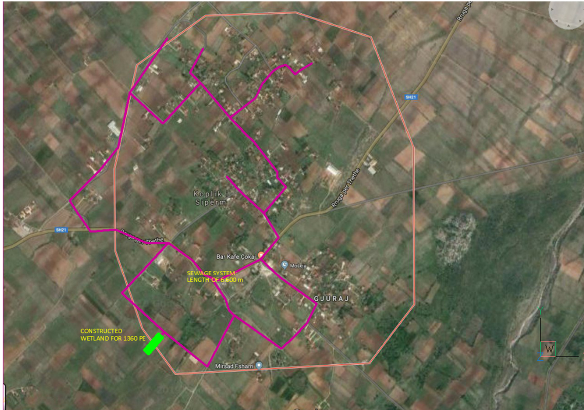
Figure 8: Scheme of the sewer system with autonomous small WWTP in the village of Koplik i Sipërm
