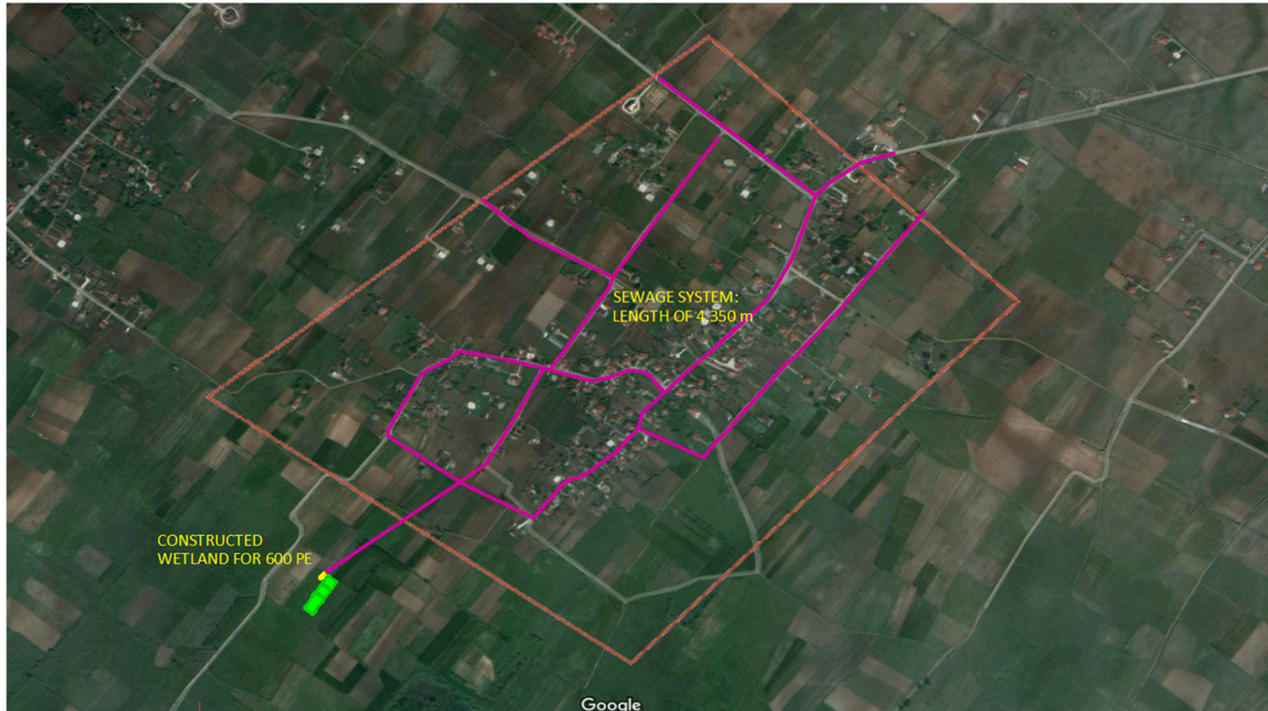
Figure 3: Scheme of the sewer system with autonomous small WWTP in the village of Kalldrun
