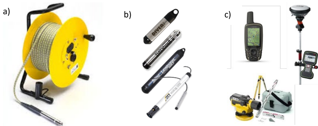
Figure 13 Field equipment for measuring groundwater heads. a) water-level meter, b) pressure sensors, and c) instruments for measuring xyz coordinates (GPS, level meter, altimeter)
