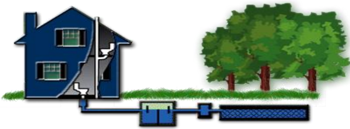
Septic tank, pipe system
