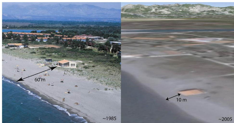
Image 7: Coastal erosion in a ten years period (~1985 - ~2005) at the Ada beach at the main delta island of Bojana-Buna in Montenegro - Source: EuroNatur, 2009
