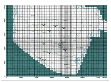
conditions have been approximated by simplified hydraulic equivalents. Eight layers were identified in the aquifer system (Table 6) from the lithological modeling which are comprised with fine, medium, coarse sand and clay. Different hydro geological parameters are assigned for each of the modelled layer (table 5).
