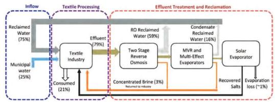
Figure 17: Reuse and reclying of waste water in industrial process
