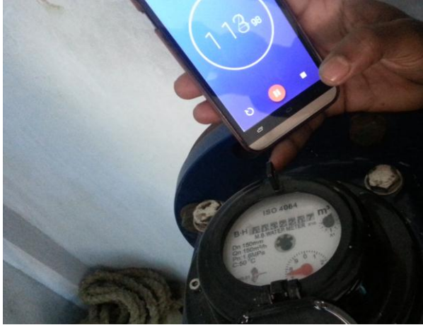
Photo 7: SIP performance verification through measurement in Doyapur SIP, Kaliganj, Jhenaidah
