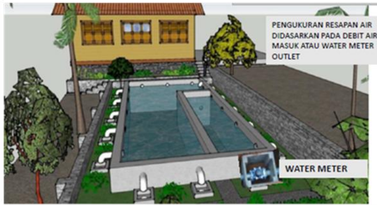
Model of infiltration pond planned on site in Indonesia language (Rohman, 2020)
