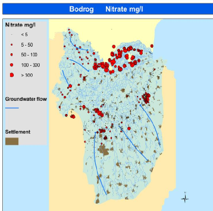
Figure 3. Nitrate concentrations in boreholes in the Bodrog-area. The blue arrows indicate the regional groundwater flow directions. Locations of settlements (brown) and numerous channels and streams into which groundwater is discharged are indicated on the background (semitransparent blue lines).
