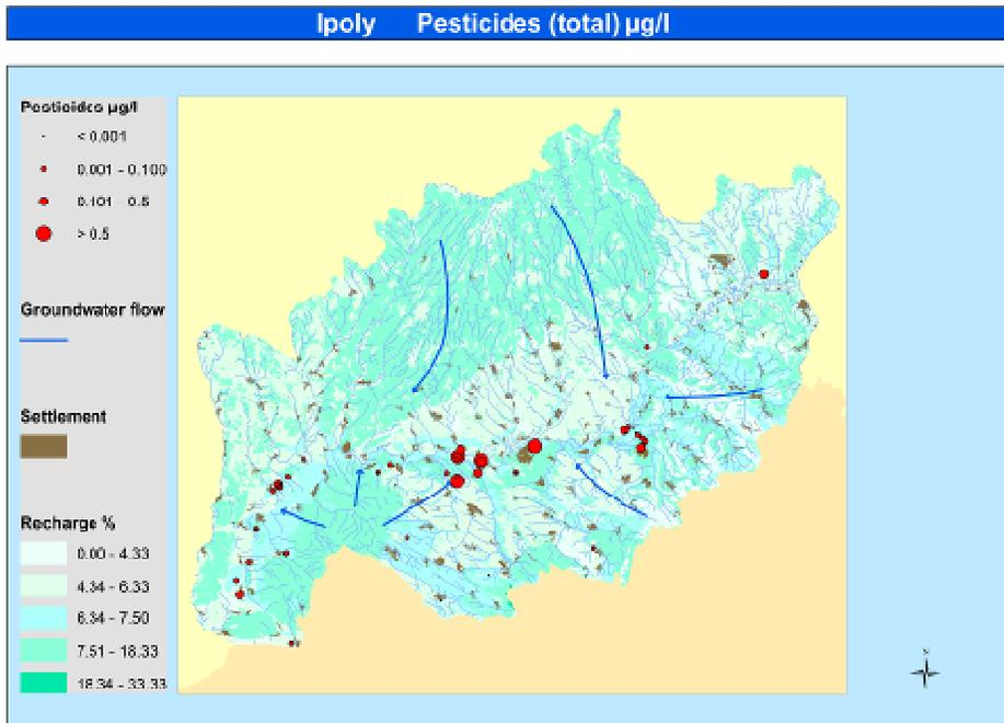
Figure 5. Pesticide sampling points scaled based on the total pesticide concentration, settlements and stream network. Blue lines indicate the regional groundwater flow directions. The background map is color-scaled based on estimated recharge distribution (Smaragd, 2008).
