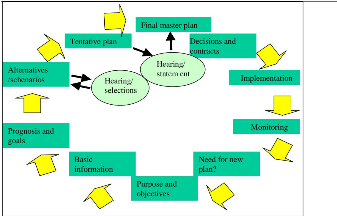
**Figure 2.** An illustration of the planning process as described in *Ympäristöopas 88 (Environmental guideline)* by Finnish Environment Institute (Vikman and Santala, 2001). The process is in principle continuous cycle the need for plan will be evaluated in 5-10 year cycles.
