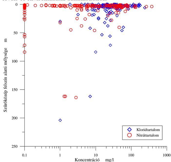
Figure 4. Changes of nitrate and chloride content with depth; Ipoly-valley.
