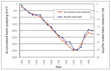
Fig. 14. Trend in cumulative withdrawals and water table in West La Mancha, 1980-2000
