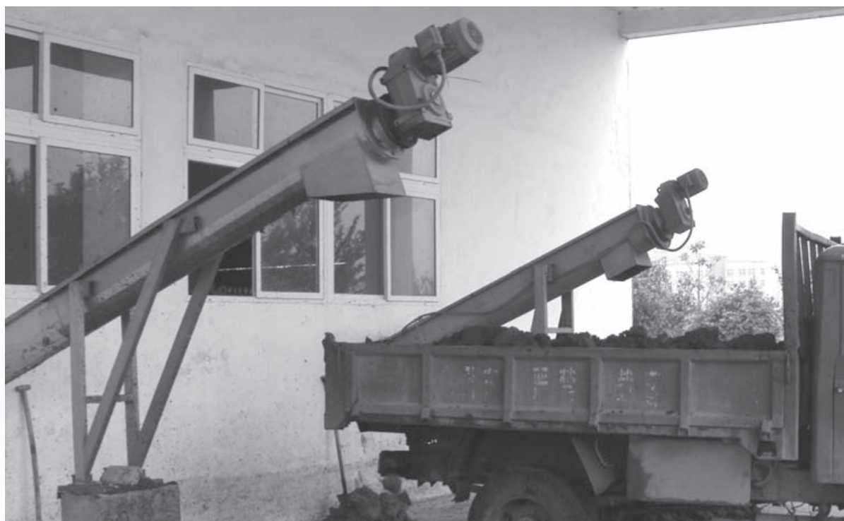
The dominant practice in the People's Republic of China is to dispose of dewatered sludge in landfills. Above, dewatered sludge being loaded for transport to the municipal landfill in Wuhan, Hubei Province. Source: AECOM 2010.
