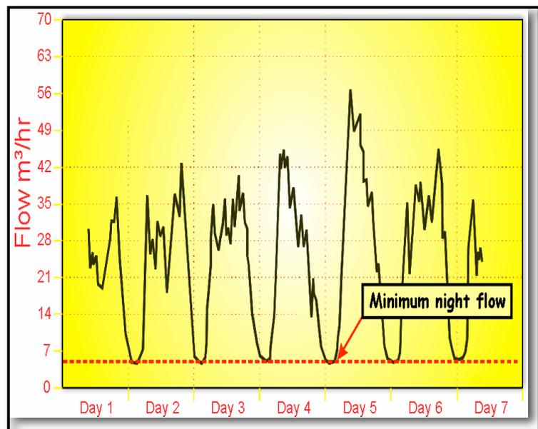
**Figure 5: Minimum Night Flow Where Leaks are Well Managed** (courtesy of Ronnie McKenzie, WRP, Ltd.)
