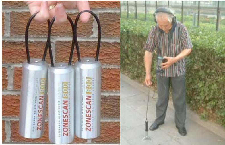
**Figure 6. Acoustic Loggers and Digital Ground Microphone for Leak Detection**
