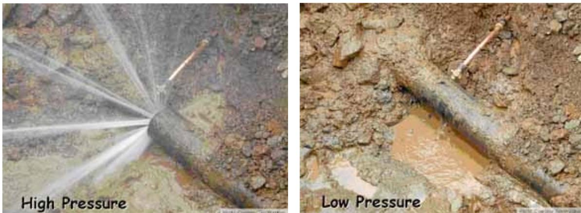
**Figure 11. Burst water main at high and low pressure**
