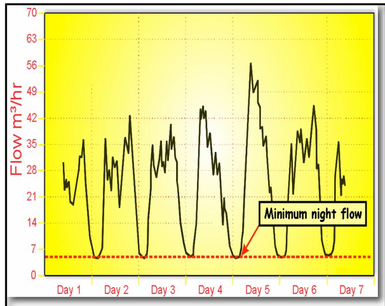
**Figure 10: Minimum Night Flow Where Leaks are Well Managed** (courtesy of Ronnie McKenzie, WRP, Ltd.)
