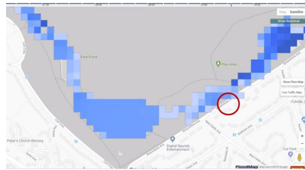
FloodMap Live forecasts show street level flood forecasts which are continuously updated using our 2D flood modelling software
