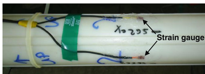
Fig. 8 Strain gauges fixed on an inclinometer casing
